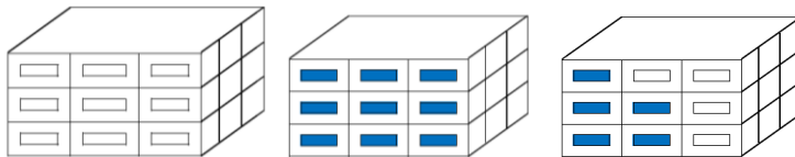
New parts only Old parts only Mixture of new parts and old parts OK Prohibited
